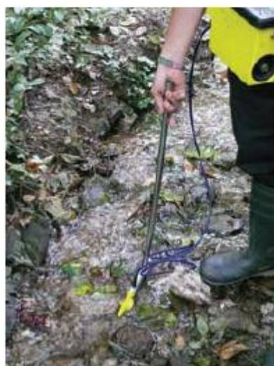
Figure 2.13 Using a flow meter to measure water speed in a forest river
