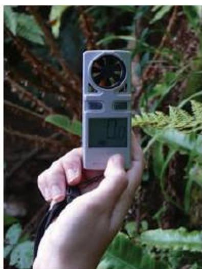
Figure 2.12 Using an anemometer to measure wind speed in a shingle ridge succession
